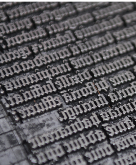
Fig. 9 (above): A printing form, consisting of movable pieces of type.
